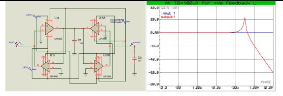
Fig. 6 4-OTA Gyrator with +Ve Feedback Simulated L & its Freq. Response graph
