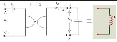
Fig. 2. Simulation of grounded inductance (L)
