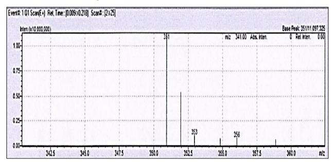
Figure 3. Formoterol D6 Parent Ion Q1 MS Q1
