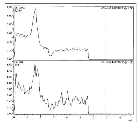
Figure 7. Representative Chromatogram of Blank Plasma
