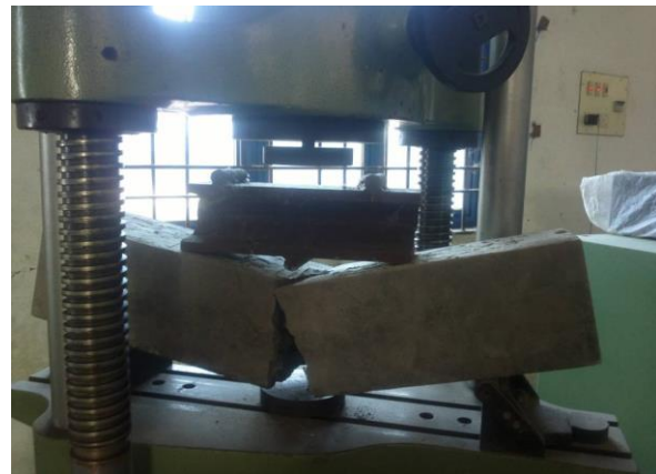
Fig 4.4 Flexural strength of prism
