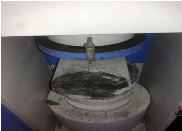
Fig 4.3 Split Tensile test on prism
