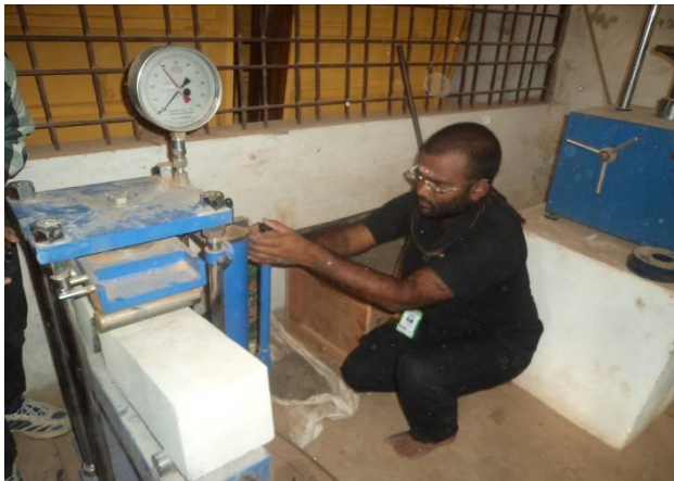
Fig 4.1 Flexural test on prism
