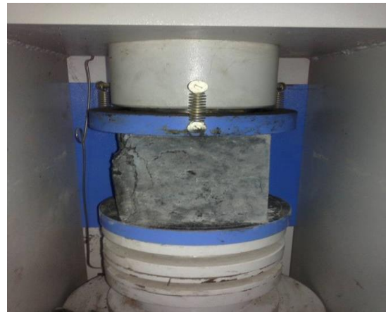
Fig 4.2 Compression test on cube
