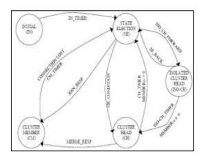
Life time of the cluster depends on the speed differences between the vehicles in the cluster. If vehicles are moving nearly same speed, then the cluster life time will be longer. Timers are maintained in controlling connections between CH and CM. If a CH does not receive any packet from CM during interval of time, CH assumes that CM has moved far and it will be detached from the cluster. Similarly CM also assumes CH has lost, if any packet is not received from CH during the time interval.
