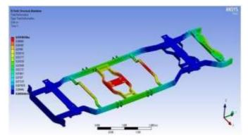
Fig. 4.8. Strain Analysis for Aluminum
