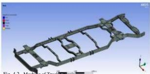
Fig. 4.2. Meshing of Truck Chassis
