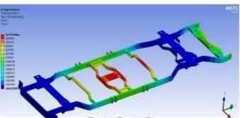
Fig .4.6. Deformation Analysis for Steel
