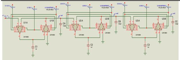
Fig.10 LC Ladder with negative fl. inductance
