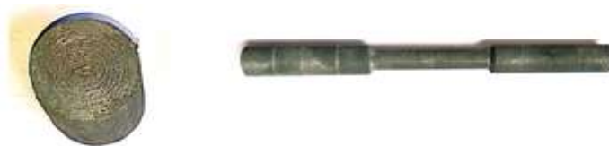
Figure 3.3 (a) Hardness Test Specimen (b) Tensile Test Specimen.
