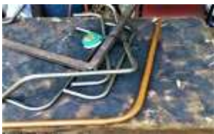
Fig 6.1 Bending of Copper Pipe
