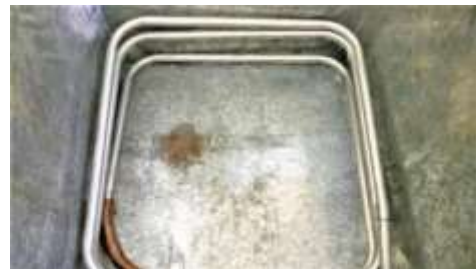
Fig 6.2 Bending of Aluminium Pipe
