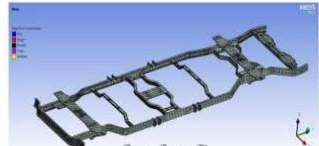
Fig. 4.2. Meshing of Truck Chassis
