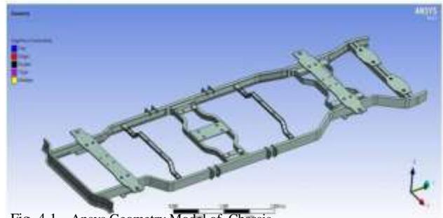
Fig. 4.1. Ansys Geometry Model of Chassis
