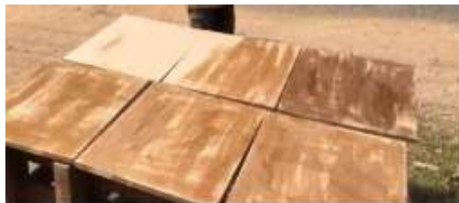
FIGURE 3: APPLICATION OF BINDER
