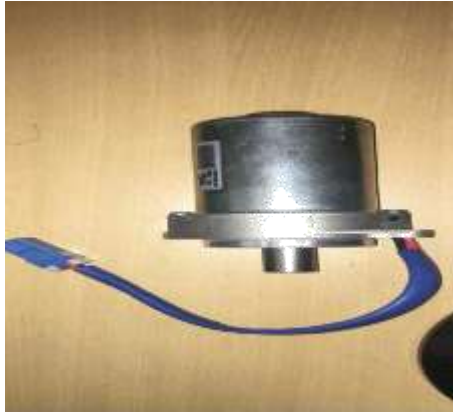
FIGURE 12: Permanent Magnet Generator
