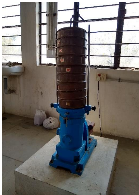
FIG NO 6: FINENESS MODULUS OF FINE AGGREGATE
