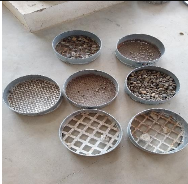
FIG NO 5: FINENESS MODULUS OF COARSE AGGREGATE
