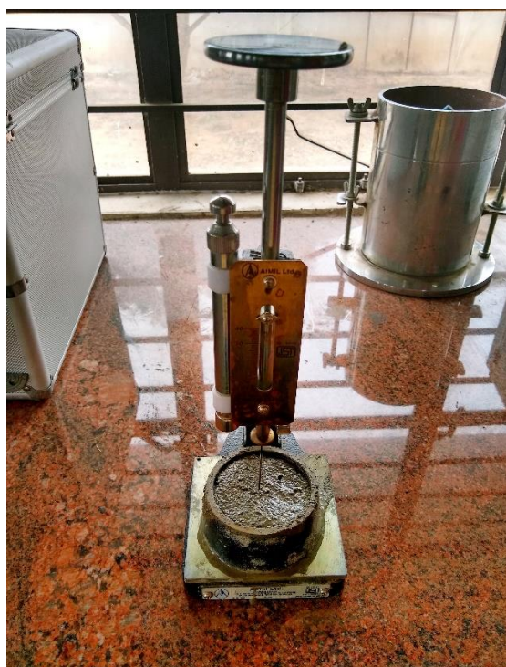
FIG NO 12: INITIAL SETTING TIME OF GGBS CEMENT
