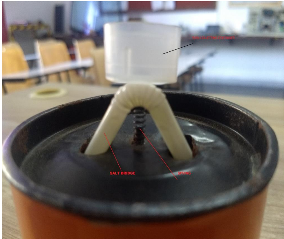
Figure 8 : Electrochemical Rain Sensor from waste materials
