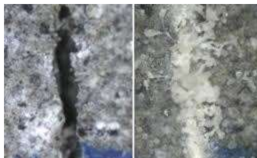
Figure -1:- Image of before and after crack by using self healing concrete
