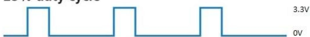
**TON:** Time required for pulse to remain ON i.e. HIGH State
