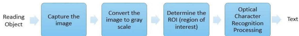
Figure 2. Flow of Detection of text using Tesseract-OCR
