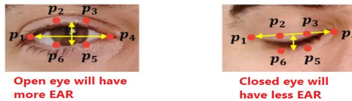
Fig 2.3 Eye Aspect Ratio Calculation
