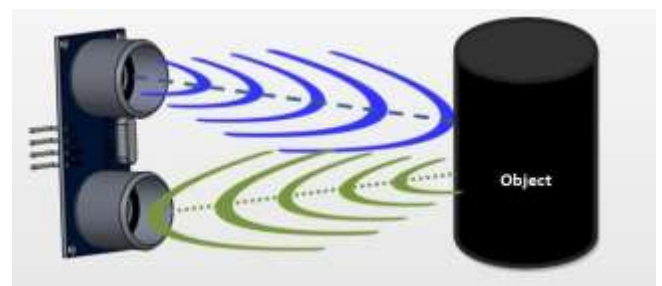
Fig.3. Ultrasonic sensor to detect human presence
