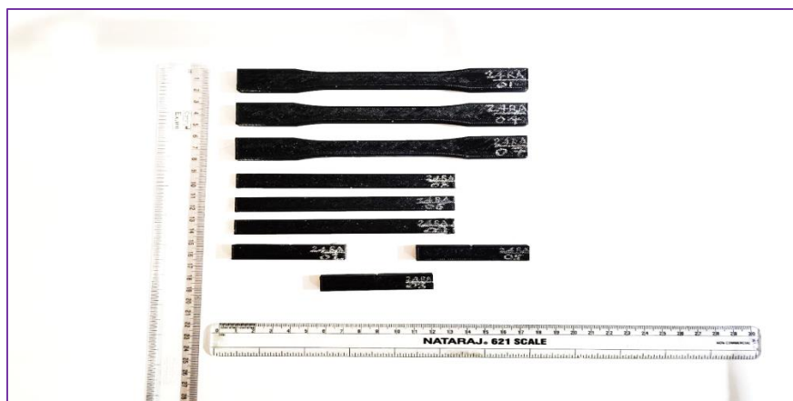
figure 2 PETG Printed Testing material
