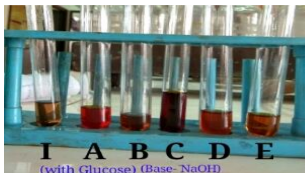
Fig. 3 Reaction of glucose with various nitro compounds; with NaOH (I); with 3,5- Dinitrosalicylic acid (A); with 2,4 -Dinitrophenylhydrazine (B.); with Nitrobenzene (C); with Picric acid(D); with m-Dinitrobenzene (E)
