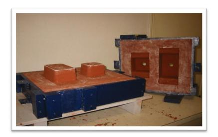
Figure 7: Mould for casting
