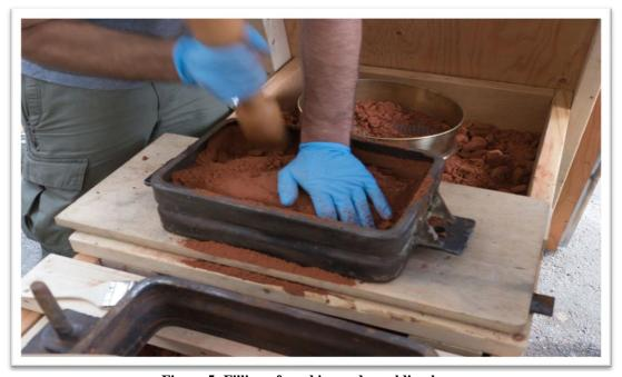
Figure 5: Filling of sand in sand moulding box.
