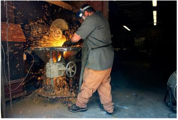
Figure 11: Trimming of excess metal
