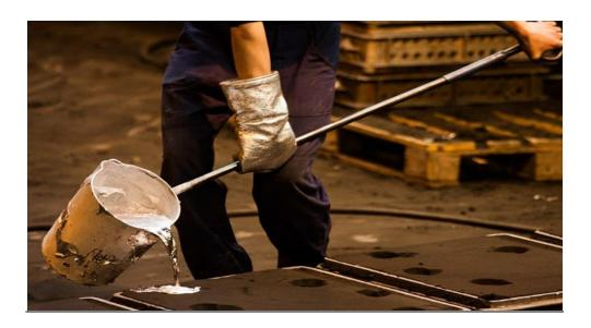
Figure 9: Pouring of liquid metal
