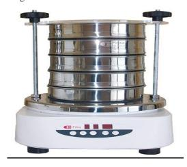
Figure 21: Standard Sieve Shaker (sifter)
