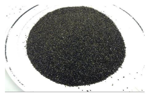
Figure 13: Sample of synthetic sand
