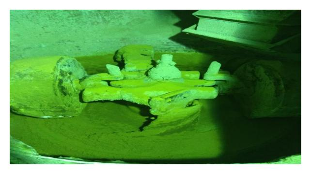
Figure 15: Mixing of binder in Moller machine
