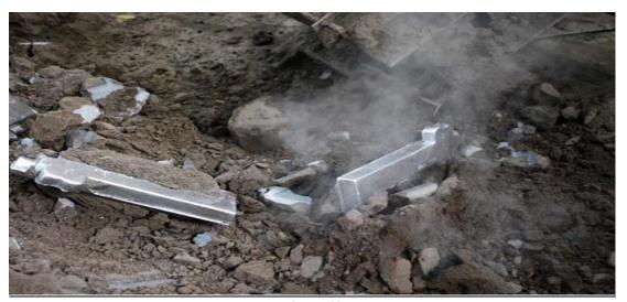
Figure 10: Broken sand mould
