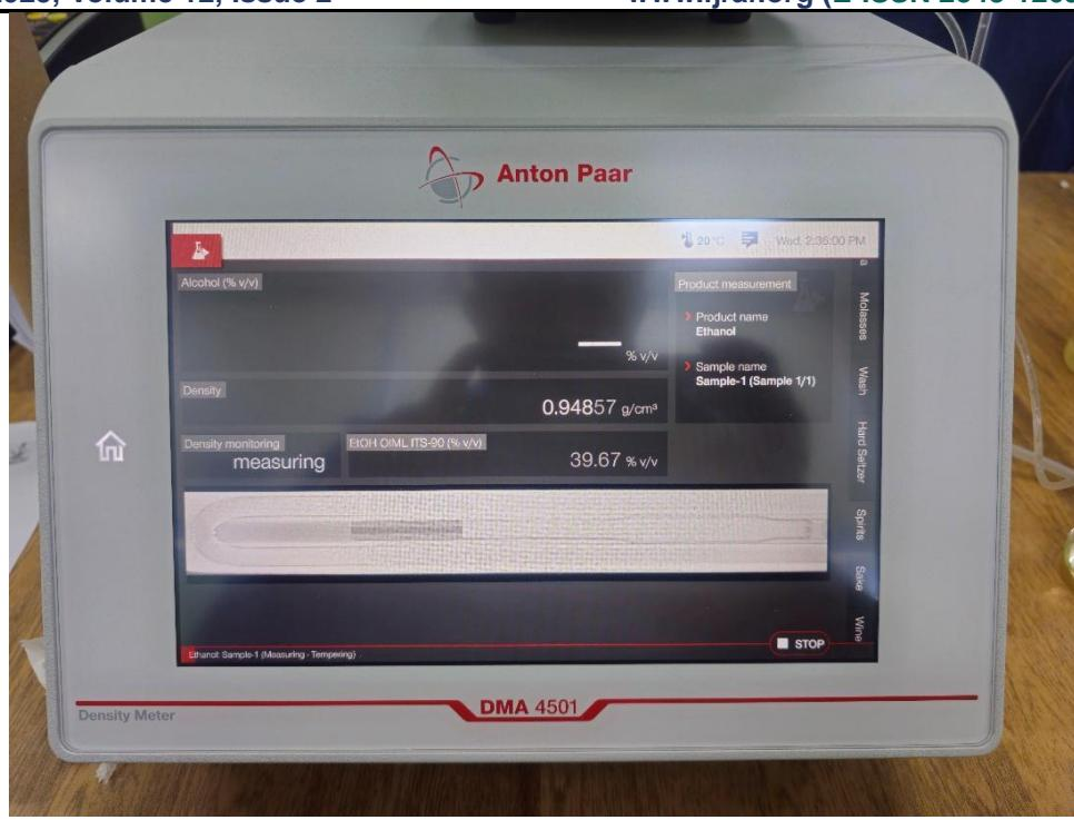
**Step 7: After that sample will be collected through the probe and the system will start measures**
