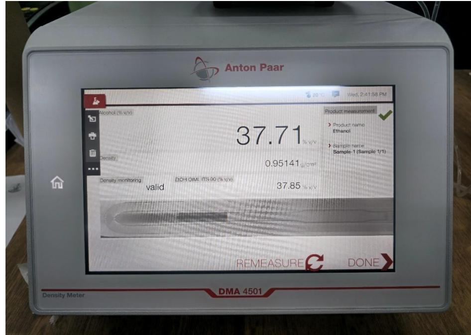
**Step 8: After the measurement the result are automatically shown on display**
