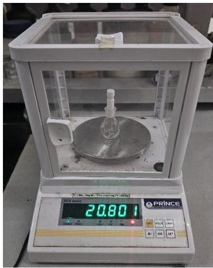
**Step 3: Weigh the empty pycnometer**
