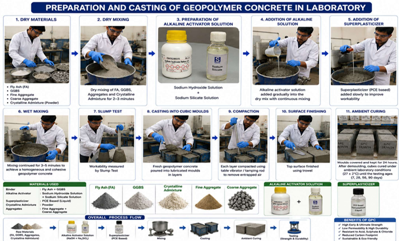
Figure 2.2: Preparation and Casting of Geopolymer Concrete in the Laboratory
