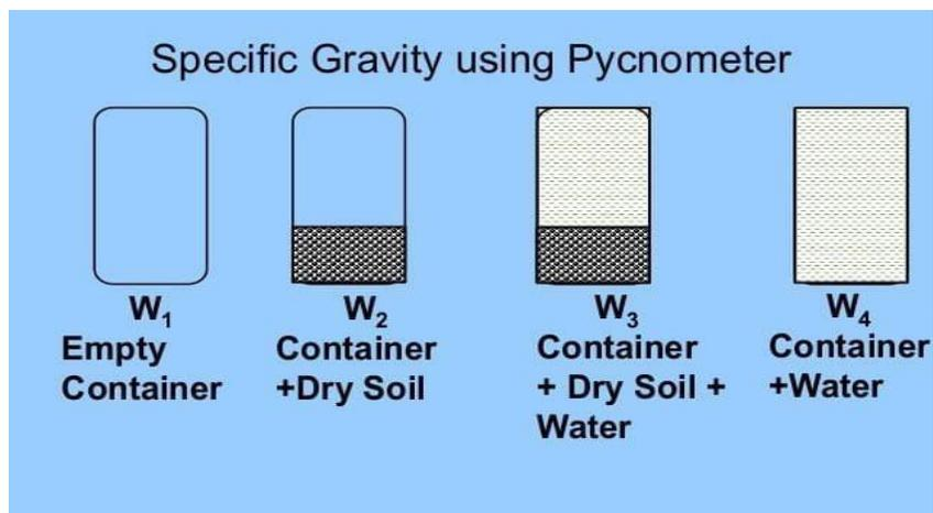
Fig:3.4.2 pycnometer measuring SG of fine aggregates
