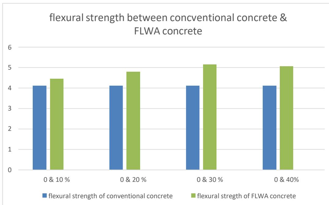
**Fig 5.1.3 Graph comparison of flexural strength between conventional concrete and FLWA concrete**
