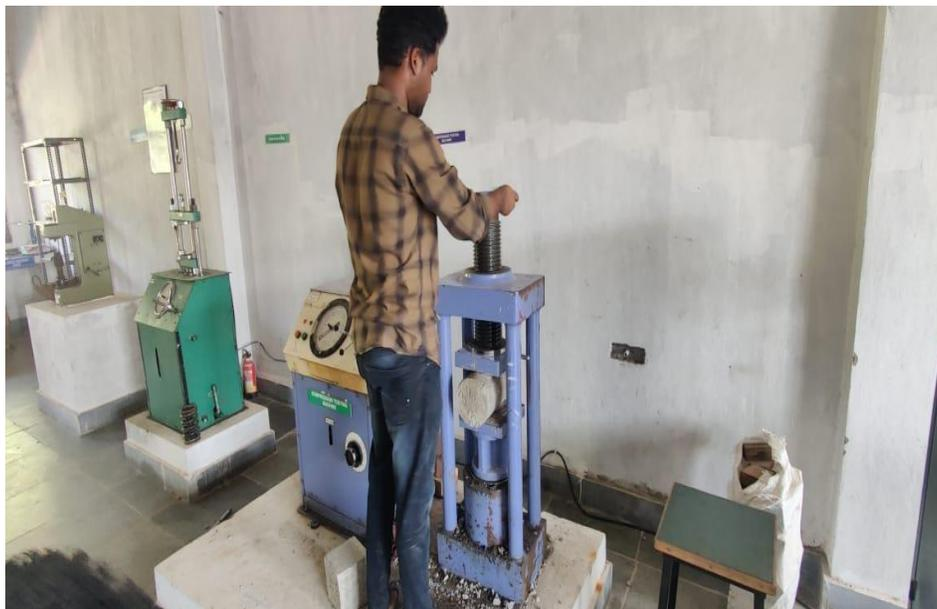
Fig: 3.8.8 cylinder in compression machine
