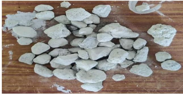
**Fig:1.2 Fly ash light weight aggregate**
