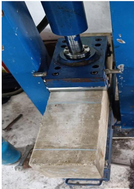
**Fig :3.8.11 beam under point load**
