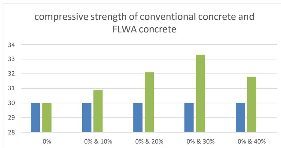
Fig 5.1 Graph comparison of compression strength between conventional concrete and FLWA concrete
