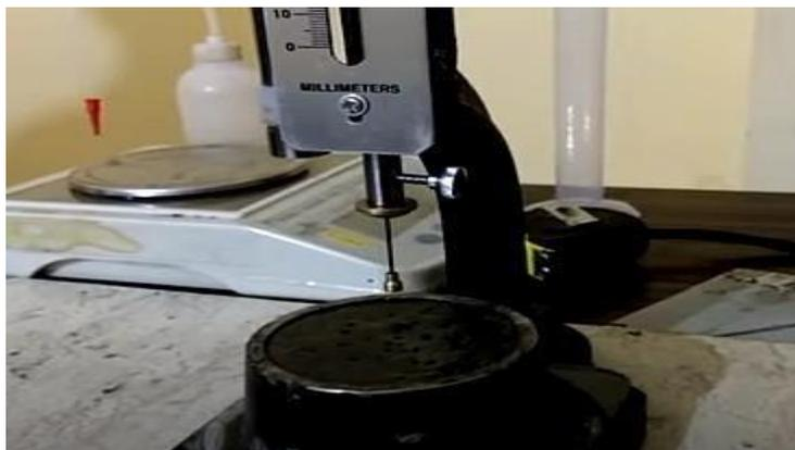
**Fig:3.3.3 Vicats apparatus for initial setting time**
