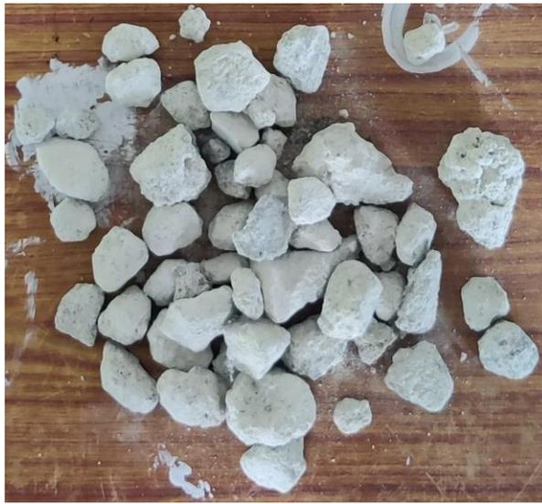
**Fig:3.2.3 Fly ash light weight aggregate**
