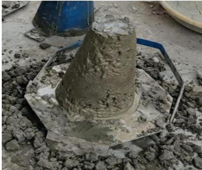
**Fig: 3.7 Slump cone**
