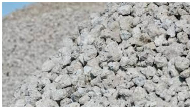
**Fig:1.1 Fly ash light weight aggregate**
