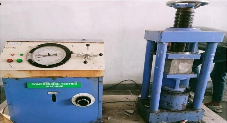
**Fig: 3.8.5** cube in compression testing machine
