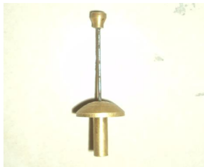
Figure 3.3 Needle for determining the final setting time of cement
