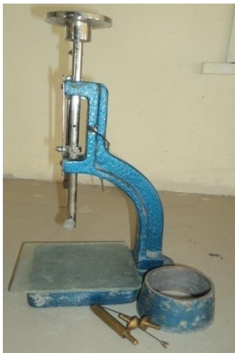
Figure 3.1 Vicat apparatus and plunger for determining normal consistency of cement
