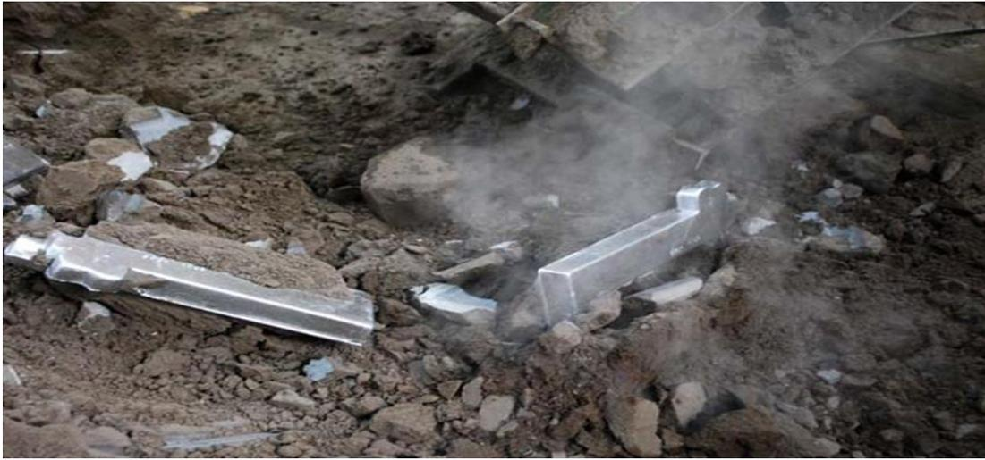
**Figure 10: Broken sand mould**
