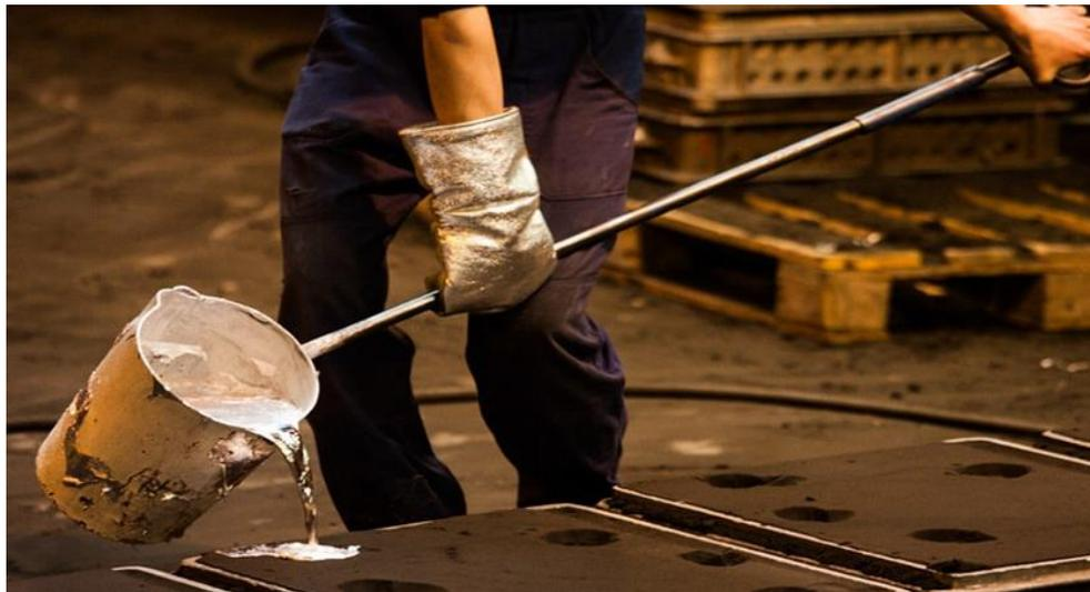
Figure 9: Pouring of liquid metal
