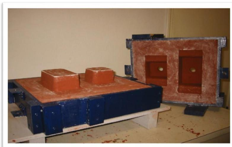
**Figure 7: Mould for casting**
