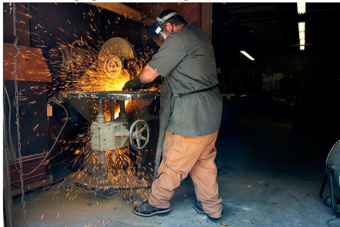
**Figure 11: Trimming of excess metal**
