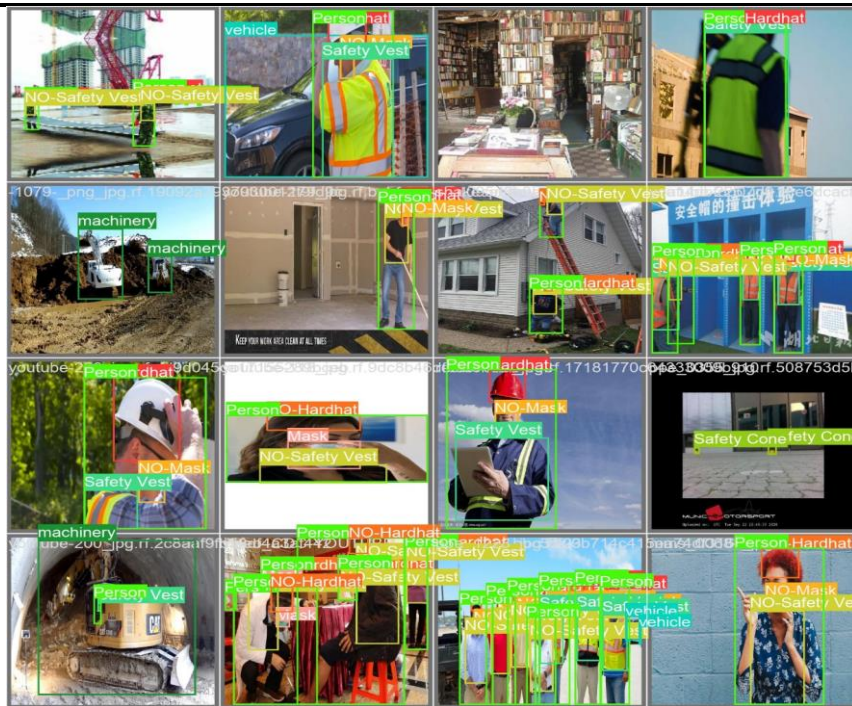
Fig. 5.3 : Picture showing the detected PPE equipments
