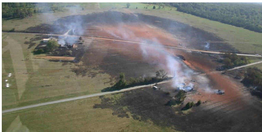
Fig 6: A view of the damage caused due to failure of a Gas pipeline. The Failure was caused due to 3 rd Party activity [Source: NTSB, USA]
