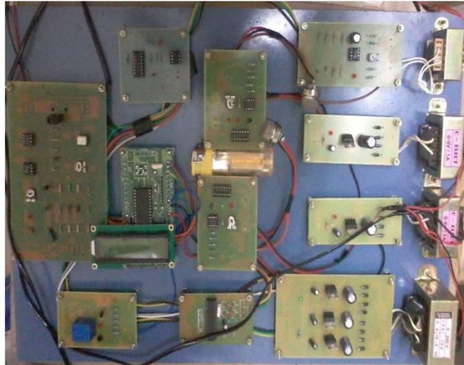
Figure.2 Photograph of wireless sensor transmitter
