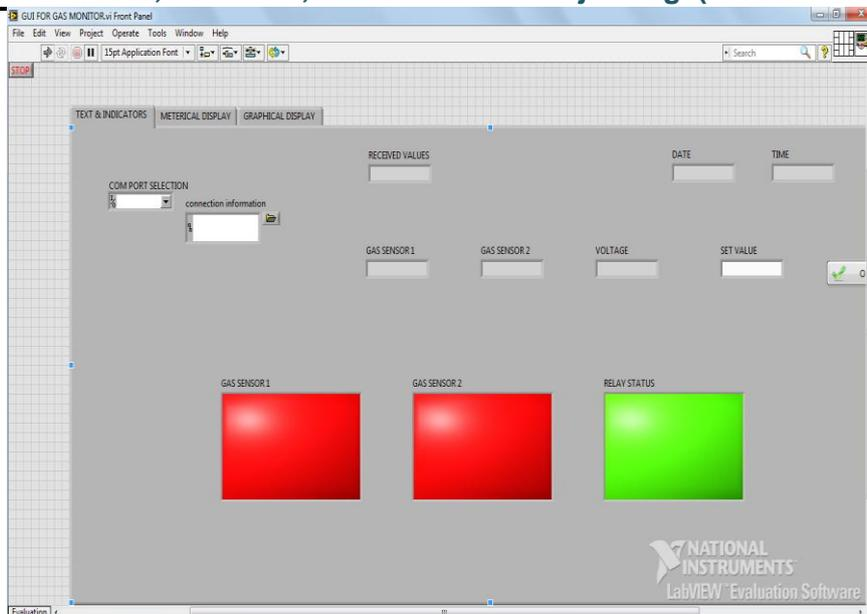
Figure.4 Front panel of gas monitoring system
