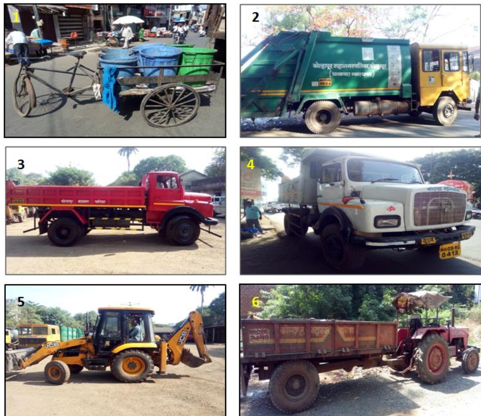
Fig. 10. KMC Vehicles (1-Tricycle, 2- RC, 3- Dumper, 4-Cargo, 5-JCB, 6-Tractor) for MSWM Activities
