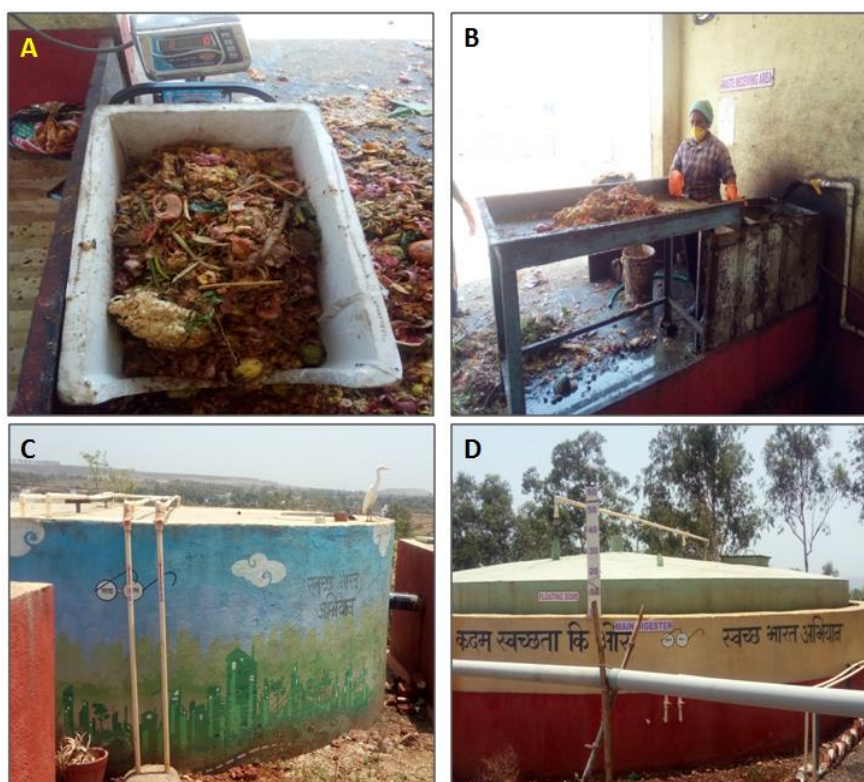
Fig. 15. A) Weighing Machine, B) Mixer, C) Small Dome and D) Large Dome
