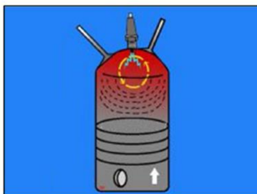
Fig.4: Tumble Flow Induction in Single Spark Ignition Engine
