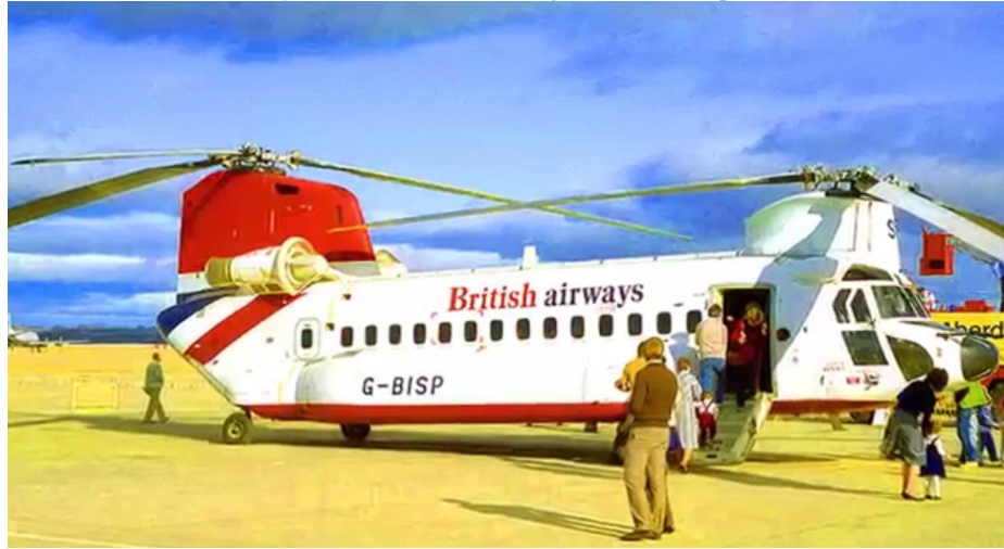
Figure 2: A tandem-rotor helicopter
