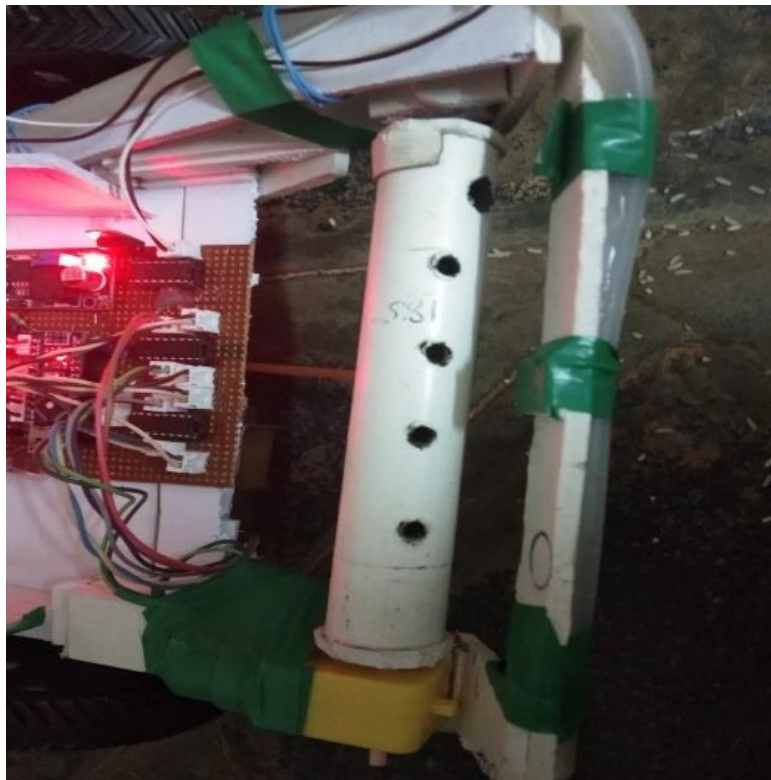
Fig.9; Seed sowing Mechanism of Agri-BoT
