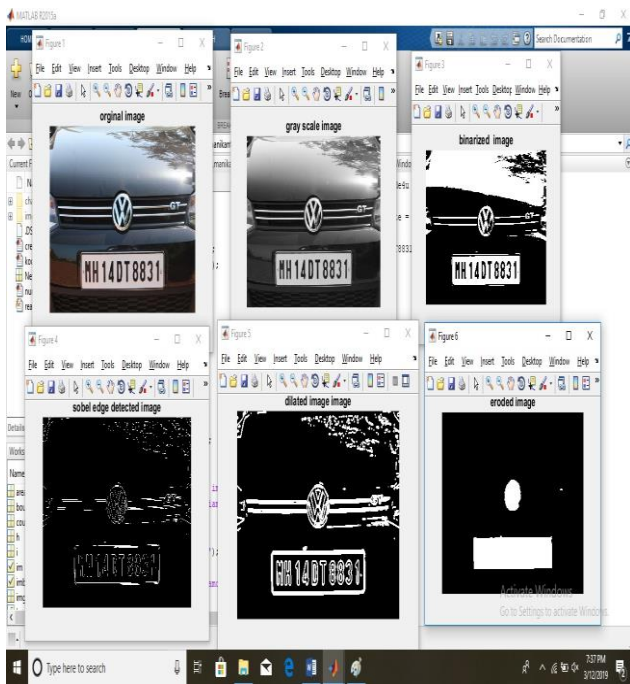
Figure: 2.6.1 Different stages in number plate extraction
