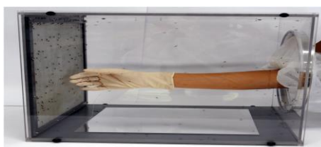
Figure no. 10: cage test for measuring the effectiveness of mosquito repellent in a laboratory
