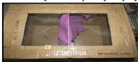
Figure no. 12: measurement of repellency by Excite-chamber test
