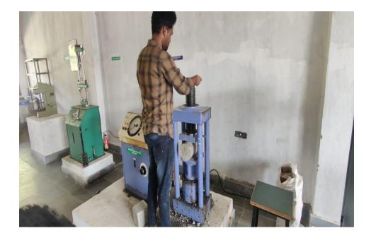
Fig: 3.8.8 cylinder in compression machine
