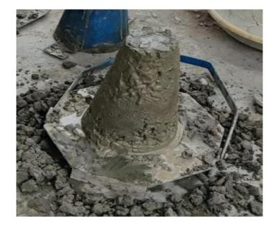
Fig: 3.7 Slump cone
