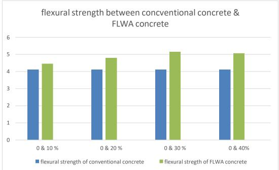
Fig 5.1.3 Graph comparison of flexural strength between conventional concrete and FLWA concrete
