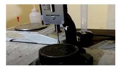
Fig:3.3.3 Vicats apparatus for initial setting time
