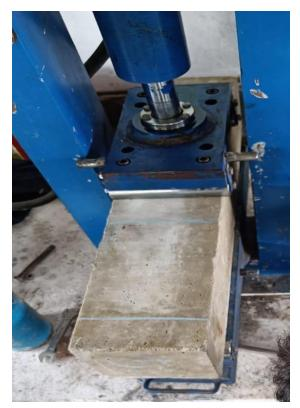
Fig :3.8.11 beam under point load
