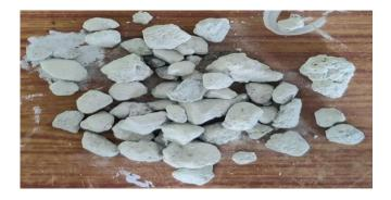
Fig:1.2 Fly ash light weight aggregate
