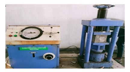
Fig: 3.8.5 cube in compression testing machine
