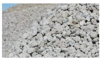
Fig:1.1 Fly ash light weight aggregate
