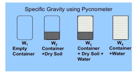
Fig:3.4.2 pycnometer measuring SG of fine aggregates
