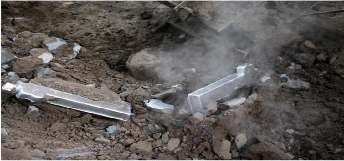
**Figure 10: Broken sand mould**
