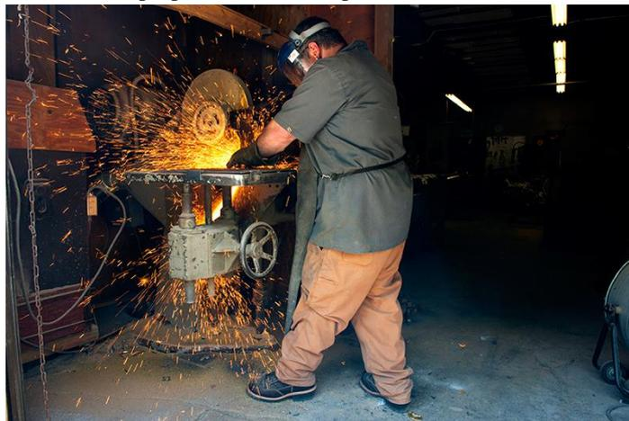
**Figure 11: Trimming of excess metal**
