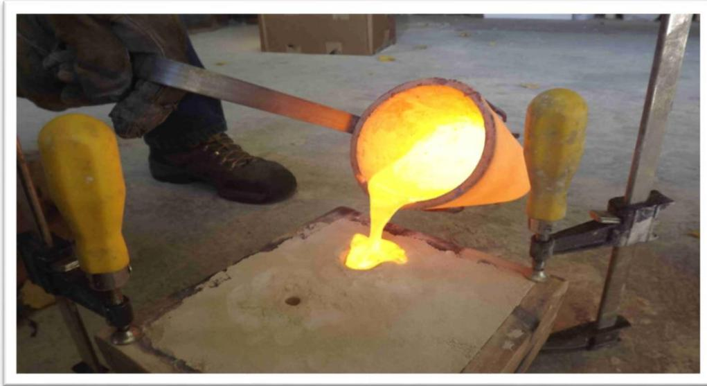
**Figure 4: Pouring of molten metal**
