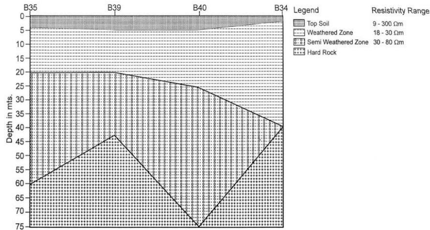
Fig. 6.5 : Geo-Electrical subsurface section from sounding data Profile - 5 Gunnempudi - Kondapalem
