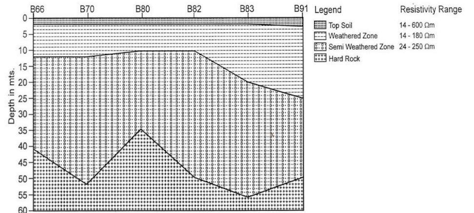
Fig. 6.8 : Geo-Electrical subsurface section from sounding data Profile - 8 Turakalapudi - Chittayypalem - China Madeena - Peda Madeena
