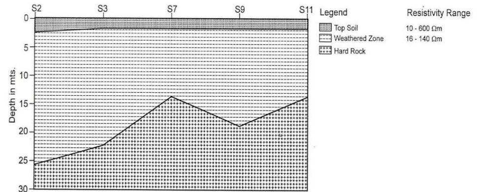
Fig. 6.2 : Geo-Electrical subsurface section from sounding data Profile - 2 Asakapalli
