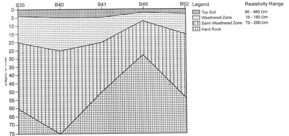
Fig. 6.6 : Geo-Electrical subsurface section from sounding data Profile - 6 Gunnempudi
