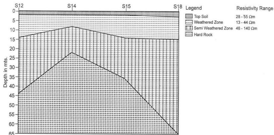
Fig. 6.3 : Geo-Electrical subsurface section from sounding data Profile - 3 Asakapalli - Pydivada
