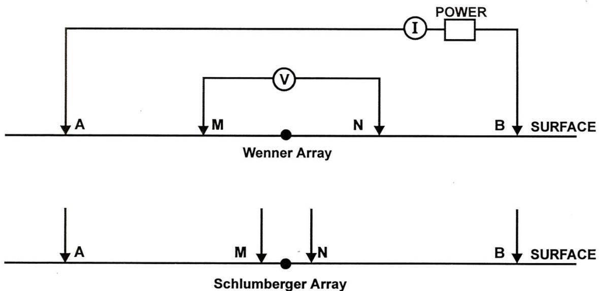
Fig. 4.1 : Diagram of Wenner and Schlumberger Arrays
