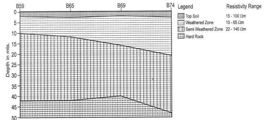
Fig. 6.4 : Geo-Electrical subsurface section from sounding data Profile - 4 Karaka, Turakalapudi, Chittayapalem, Taipuram
