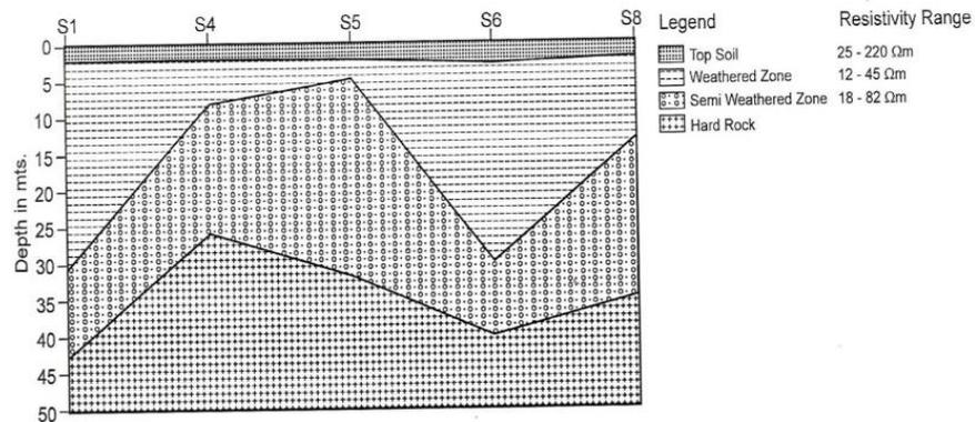
Fig. 6.1 : Geo-Electrical subsurface section from sounding data Profile - 1 Asakapalli
