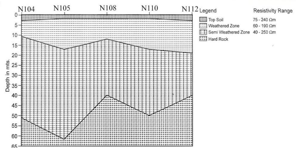
Fig.6.10: Geo-Electrical subsurface section from sounding data Profile - 10 Karaka
