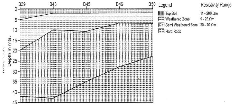
Fig. 6.7 : Geo-Electrical subsurface section from sounding data Profile - 7 Gunnempudi
