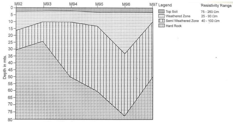
Fig. 6.9 : Geo-Electrical subsurface section from sounding data Profile - 9 K. Vallapuram
