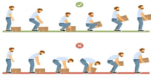
Fig. No. 14 Safe and Unsafe Practice in Manual Materials Handling
