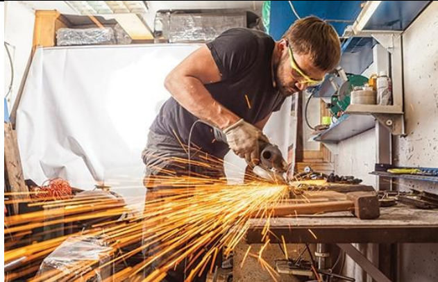
Fig. No. 13 Fire Hazard During Grinding Operation
