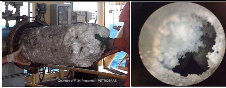
Fig.2.4: hydrate plug in subsea pipelines/ flow lines
