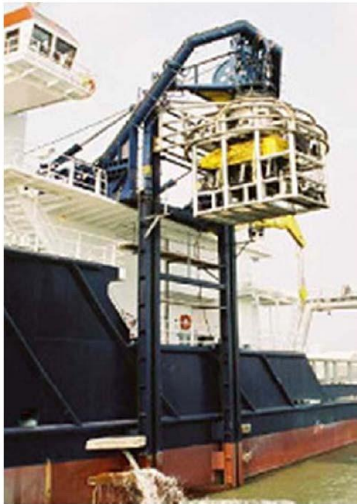
Figure 33: Guide Rail System
