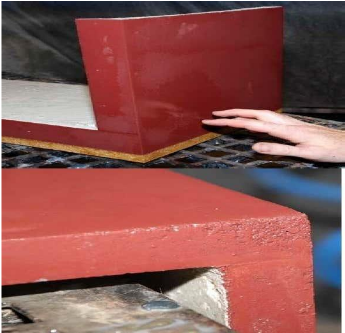
Fig. Sand buildup in corner
