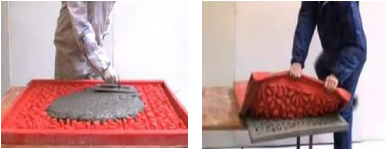
Figure 3. Pre-mixture and casting process
