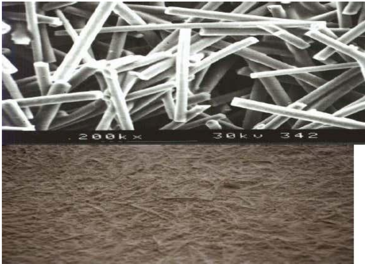
Fig. 2D reinforcing with Glass fiber
