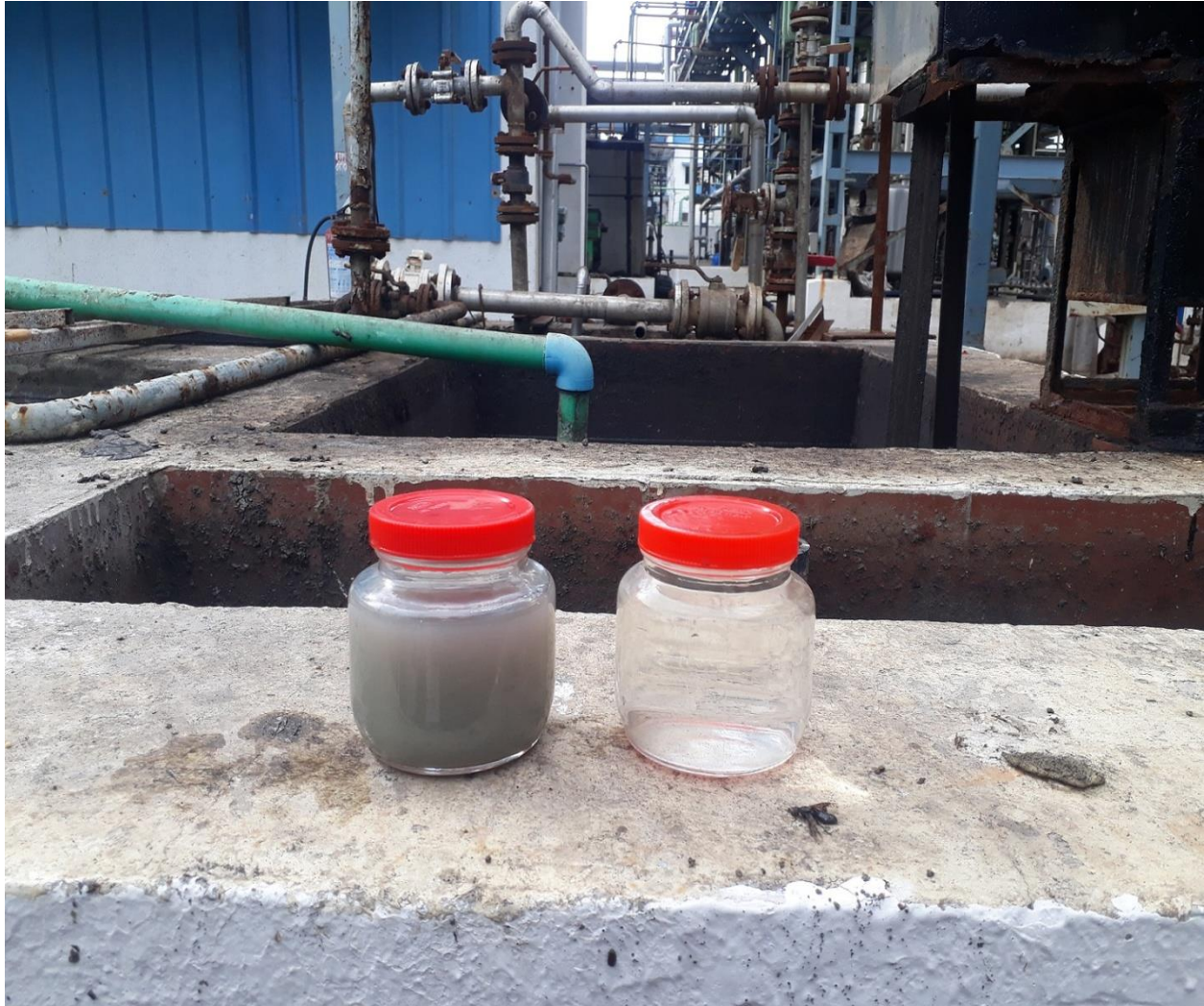
Fig: ETP INLET & OUTLET SAMPLE
