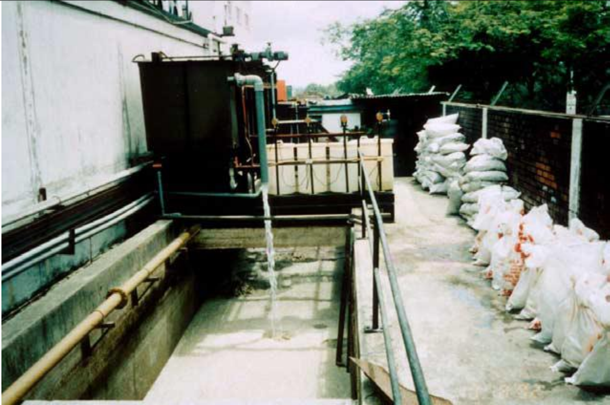
Fig. 4.4.2. Coagulant assisted DAF (top LHS) treating milk canning wastewater.
