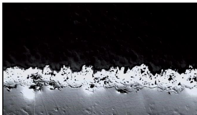
Fig 43. Porous surface in the range of TPS (150 to 400 \mu\text{m} )
